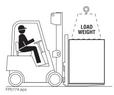
Load weight must not exceed combined truck/ attachment capacity (see truck nameplate).
