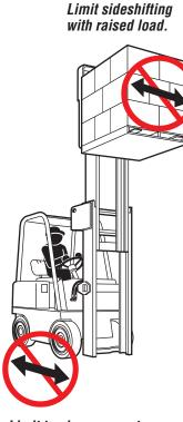
Limit truck movement with raised load.
