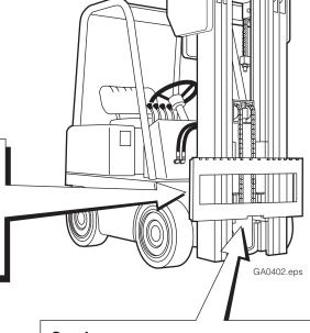
**Carriage** – Clean and inspect carriage bars. Bars must be parallel and ends flush. Grind smooth any protruding welds that may affect lower hook engagement. Repair any damaged notches.
