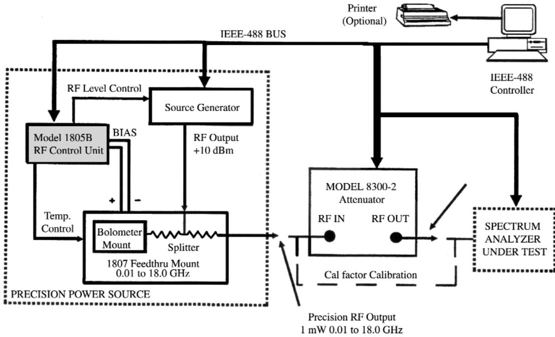
Figure 1-8 Spectrum Analyzer Calibration Setup
