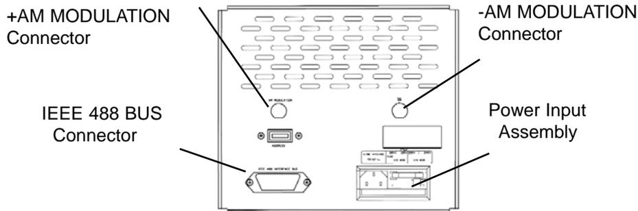
**Figure 2-3 Model 1805B Connector Location (REAR)**
