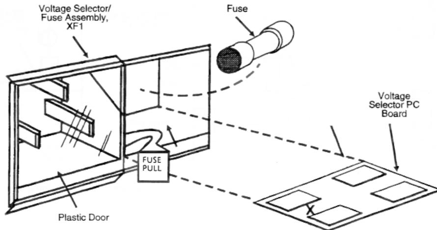
**Figure 2-5 Voltage Selector/Fuse Assembly**
