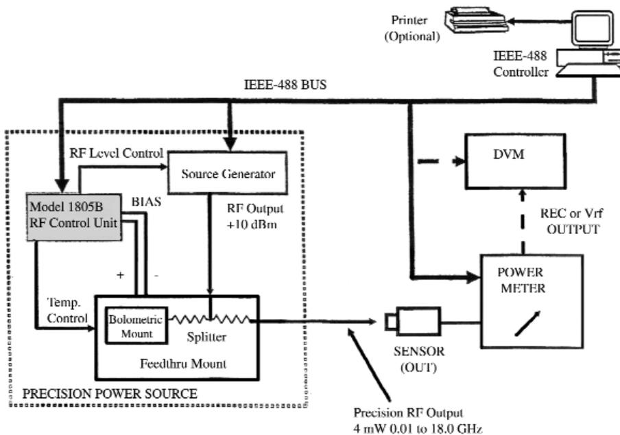
Figure 1-3 Typical Coaxial Power Sensor Configuration
