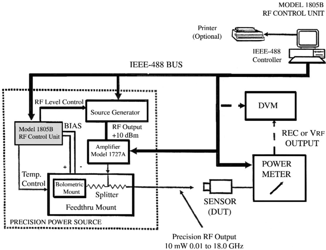
Figure 1-4 10 mW Configuration Using Model 1727A
