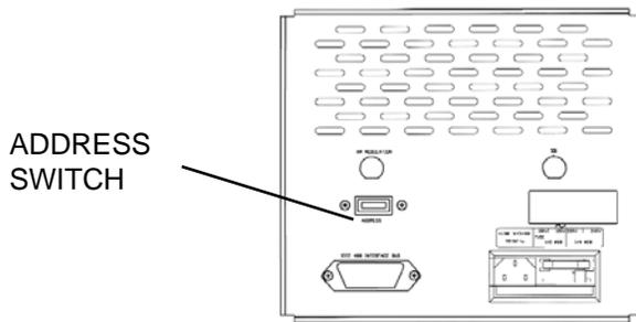
**Figure 3-2 Controls and Indicators (Rear)**
