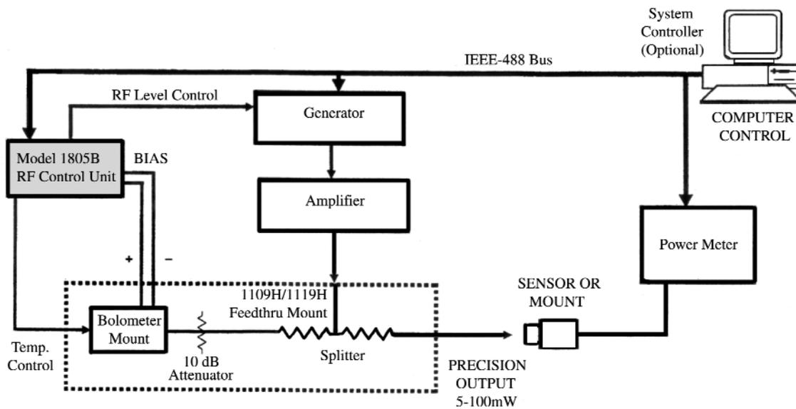
Figure 1-7 Typical Higher Power Calibration Setup
