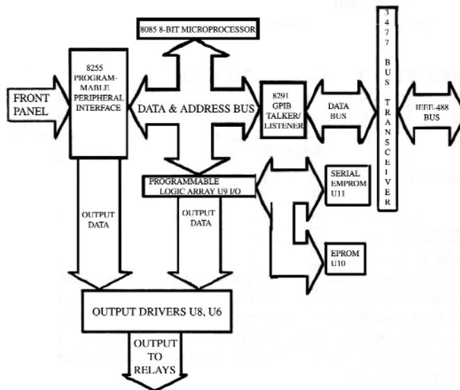
Figure 3-4 Simplified Microprocessor Block Diagram
