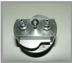
Valve head of the floating piston cylinder (FPC)
