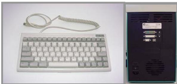
On the rear panel of the instrument you find a connector for a PC-keyboard (Please use an IBM PC-AT or compatible keyboard). A keyboard with protection cover can be ordered from GRABNER INSTRUMENTS directly. Connect the keyboard.
