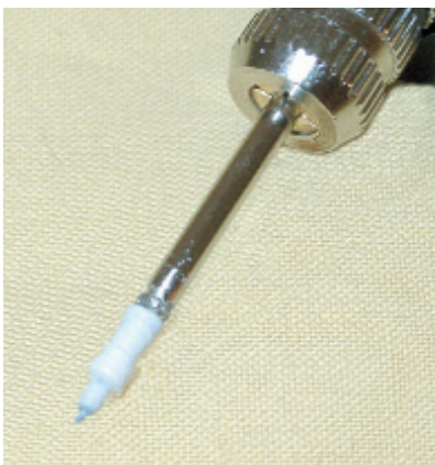
Fig.1. High drill speeds and most plastics do not go well together
