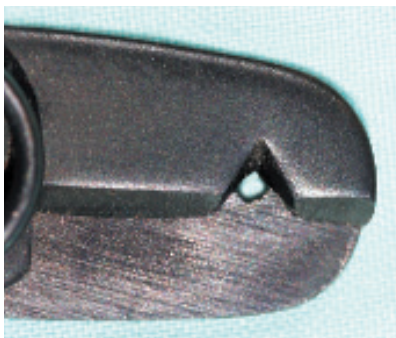
Fig.3. The notched blades of wire strippers should prevent damage to the wires
