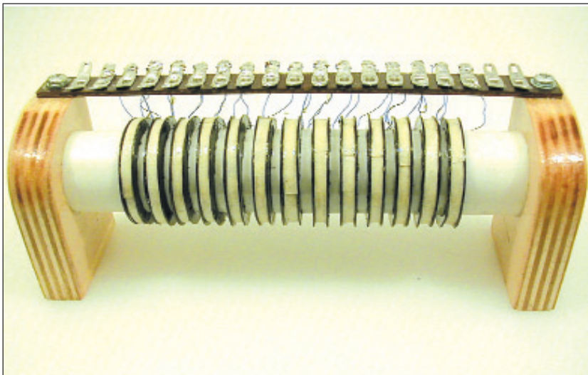
Assembled LF/VLF aerial-to-receiver matching tapped inductor coil
