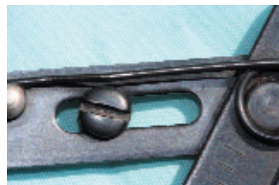
Fig.4 Loosening the bolt enables it to be slid to a new position and tightened again. This method of adjustment is fine if only occasional readjustment will be needed
