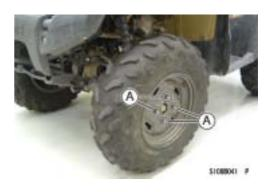
• Lift up the front wheels and remove the wheel nuts and wheels.
