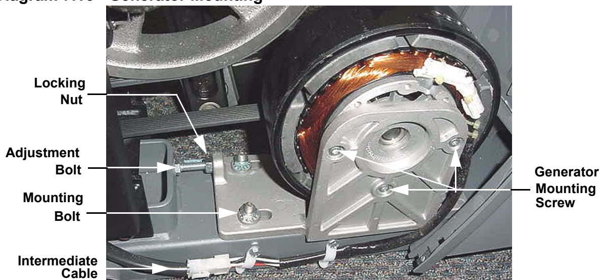
Diagram 7.16 - Generator Mounting
