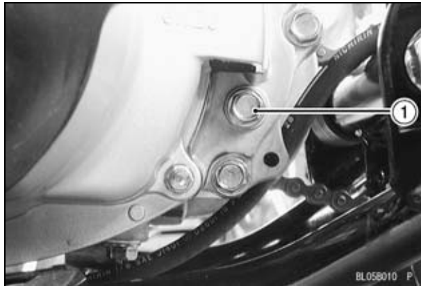
1. Oil filler bolt/measurement hole
