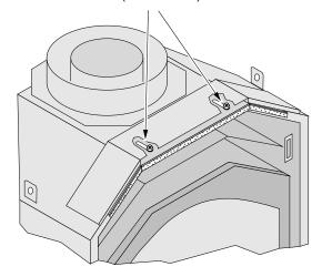
Slide the heat shield forward until it is flush with the facing and tighten the nuts to secure.
