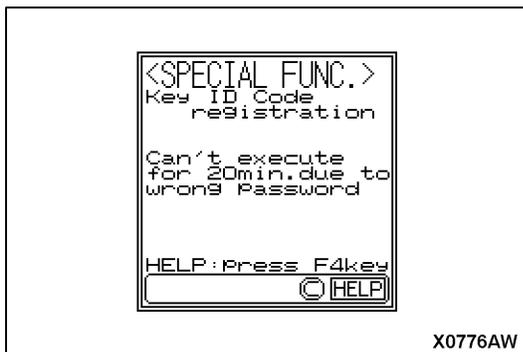
3. If an incorrect password is input five times in a row, this screen is displayed and the immobilizer-ECU switches to "Unauthorized operation, start-prevention mode."
