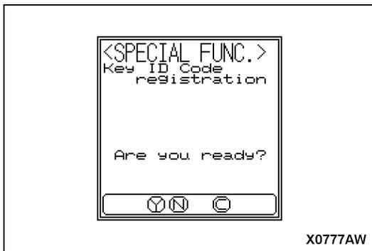
4. Insert the key to be registered into the ignition switch. Turn the ignition switch to the "ON" position. Press the "YES" key to start key ID registration.
