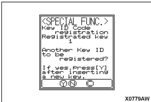
6. The number of keys currently registered will be displayed. To register an additional key, replace the ignition key with the next key to be registered within *five seconds* and then press the "YES" key. Press the "YES" key. Key ID registration screen will be displayed, then register another key.
