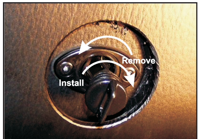
Figure 5-2. Removing and Installing the drain plug.
