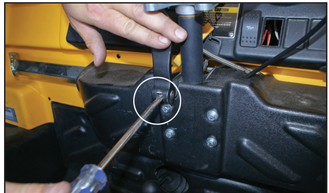
Figure 3-3. Adjustment on cam lever.
