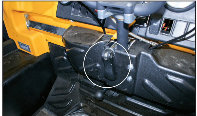
Figure 3-2. Steering position adjustment.
