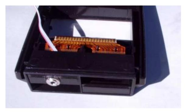
**13.** Route the cable down the side of the calculator body, between the edge of the battery compartment and the outside of the case. It is helpful to use double-sided tape to hold
