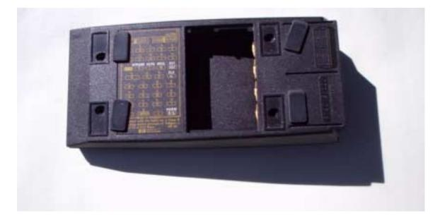
**6.** Lift off the bottom case and the U-shaped center case section. Note the orientation (front-to-back) of the center case section, because it not symmetric.
