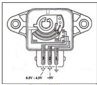
Figure 1.2: TPS Pinout
