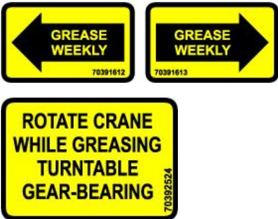
Crane worm gear bearing teeth must be lubricated weekly with Molub-Alloy 936 or equivalent, applied with a grease gun or brush. Cover all teeth with grease and leave no exposed metal surfaces showing.
