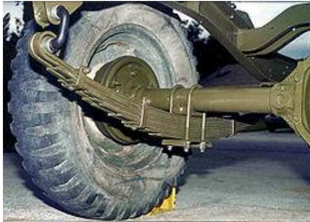
Fig 2: Leaf spring fitted in a vehicle
