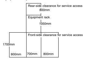
2. If the server is installed at a level between 21U and 40U (\*1): (\*1 Judged based on the level of the equipment top)
