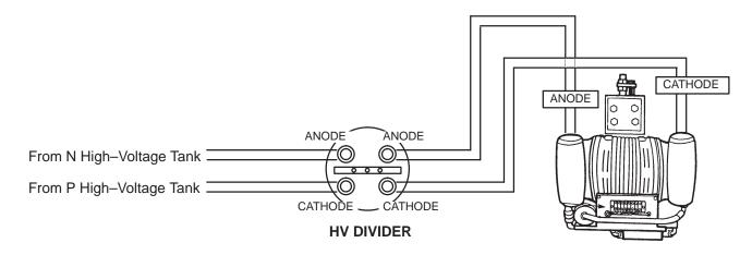
10. Select the multimeter to the voltage mode and connect the probes to the HV divider's terminal corresponding to anode and ground.
