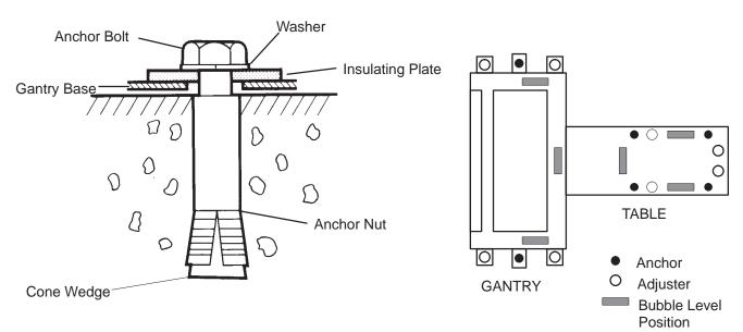
2. Verify that the Gantry is in no contact with the floor. If not, adjust feet for isolation.
