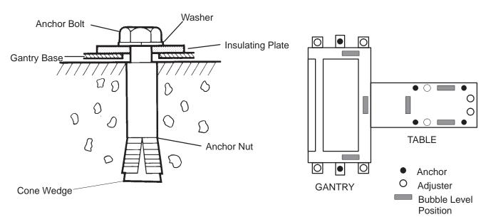
2. Verify that the Table is in no contact with the floor. If not, adjust feet for isolation.
