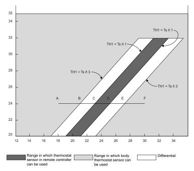
Example: Assuming the preset temperature above is 24°C, and the suction temperature has changed from 18°C to 30°C (A --> F):
