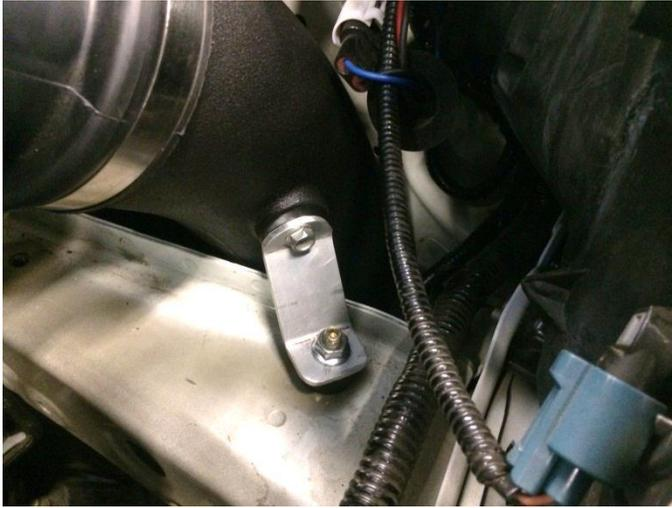
10. Extend the wires for the MAF sensor. Take the ten wire connectors and five 12" strips of wire and extend the five wires for the MAF sensor. Use electrical tape to cover wires after you are finished. Connect to MAF sensor.
