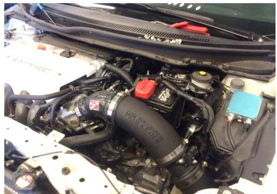
9. Install Support Bracket. Install supplied isolator into frame, install bracket onto isolator and secure bracket to isolator with the supplied nut. Install supplied 10MM bolt into lower intake tube.
