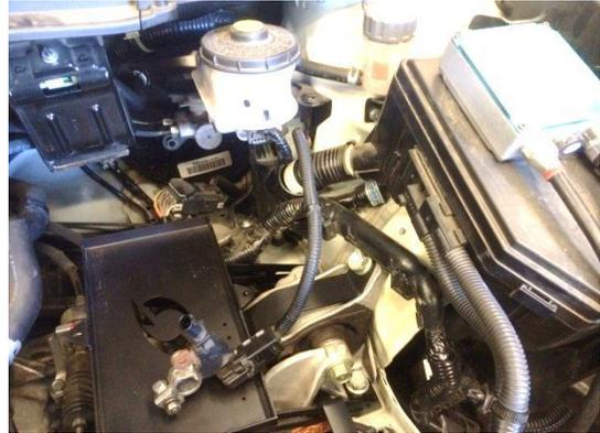
4. Install the battery in the newly mounted battery relocation bracket and secure it with the factory tie down. Secure the negative (-) battery terminal to the battery.
