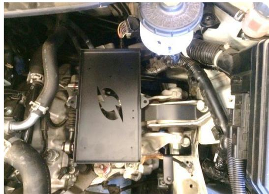
3. Relocate the negative (-) terminal with 10MM bolt to its new location on the brake master cylinder bracket on the driver side shock tower.
