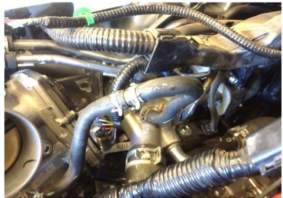
8. Install coupler on to throttle body with two clamps, install upper intake pipe, install MAF Coupler with two clamps, install lower intake pipe, and secure air filter using clamp.
