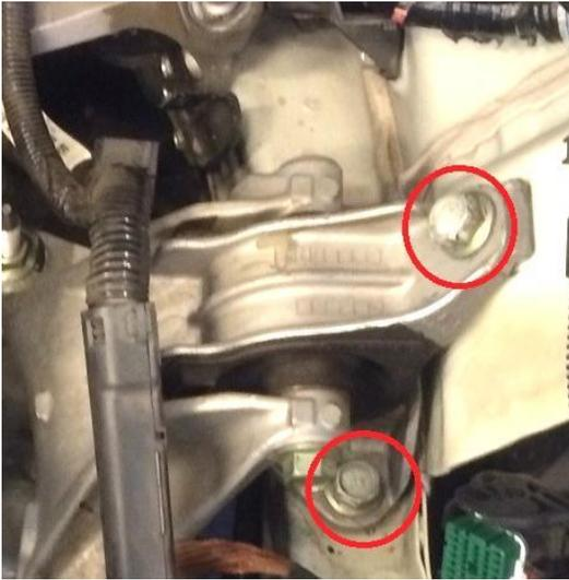
2. Install the battery relocation bracket onto the engine mount and reinstall the three factory transmission mount bolts and torque to factory specs.
