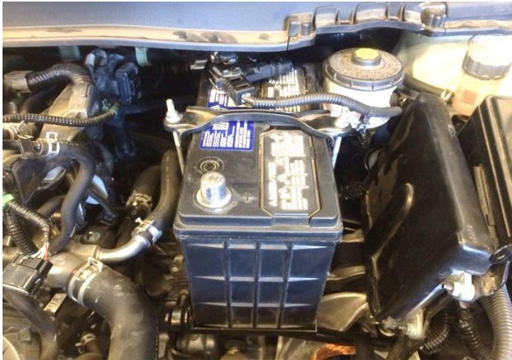
5. Extend the two wires from car harness to the negative (-) battery terminal. Use the four supplied wire connectors and the two supplied 18" long strips of wire. Use electrical tape to wrap connections after you are finished. Route up around fuse box to battery.
