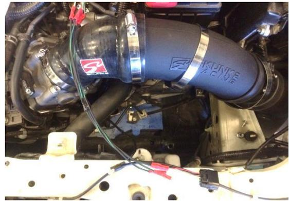
11. Use the supplied 1/2" hose to connect the valve cover breather to the intake tube. Secure hose with the two supplied zip ties.
