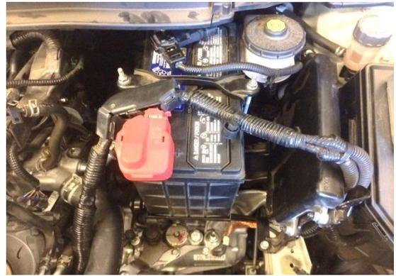
7. Remove factory breather tube that connects the valve cover to the intake tube. There are two coolant lines connected to the tube. Use the supplied brass 5/16" connector to connect the two hoses together.
