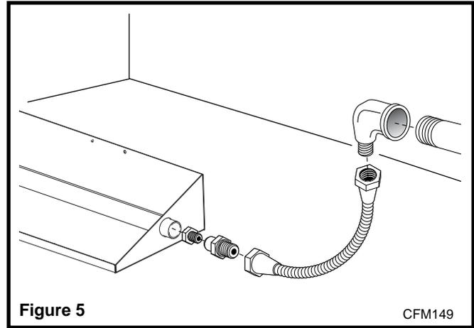
**Remember to use pipe thread sealant or teflon tape only on the straight pipe threads. Do not use any on flared ends.**
