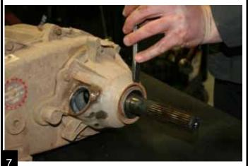
Remove the rear output shaft snap ring.
