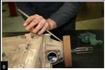
Remove the rear output shaft seal.
