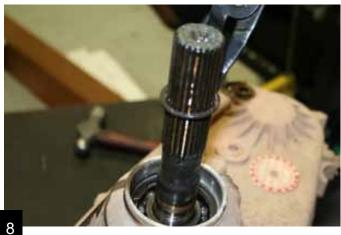
Remove the 5 bolts holding the tail housing in place. Separate it from the transfer case.
