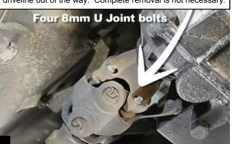
Remove the front output yoke.
