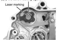
1 1 . Place the spring in the stopper arm, fit them into the stopper plate on the case, and tighten the bolt to the specified torque.
