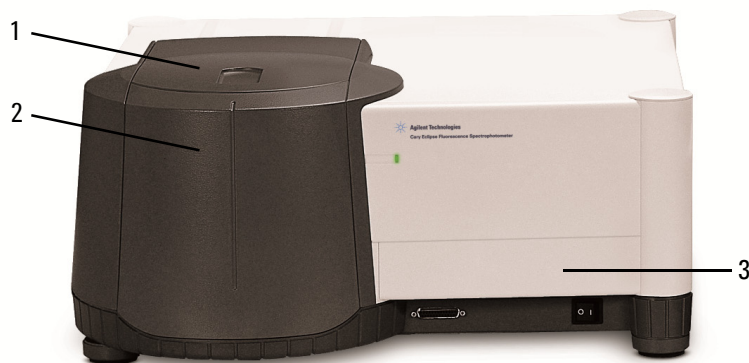
Figure 1. Cary Eclipse showing the sample compartment lid (1) and front panel (2) and Lamp Access Panel (3)
