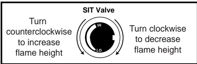
Fig. 22 Flame adjustment knob for SIT Valve.
