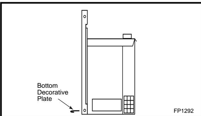
Fig. 45 Slide bottom decorative plate under unit floor.
