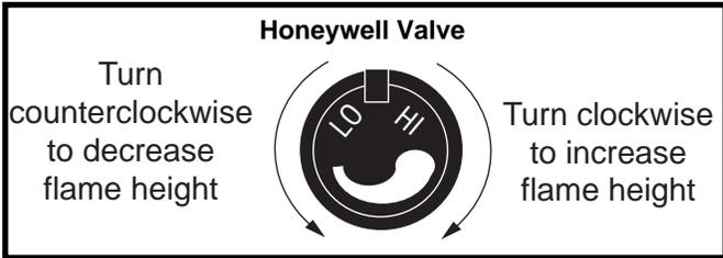
Fig. 21 Flame adjustment knob for Honeywell Valve.
