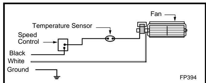
Fig. 4 Wiring diagram.
