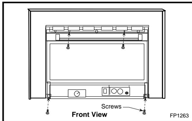
Fig. 41 Frame mounting.
