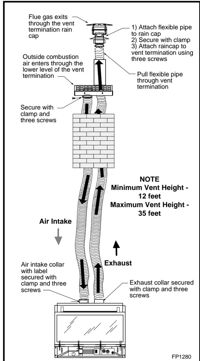
**Fig. 9** Liner installation.
