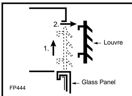
Fig. 16 Louvre removal.
