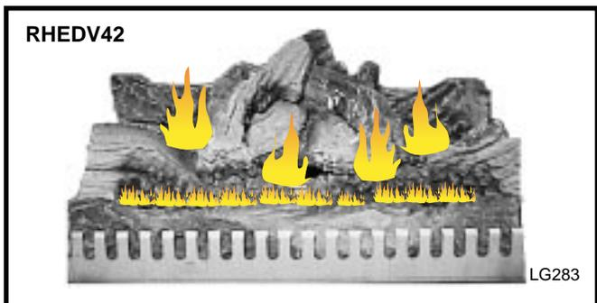
Fig. 26 Correct burner flame appearance for RHEDV42.
