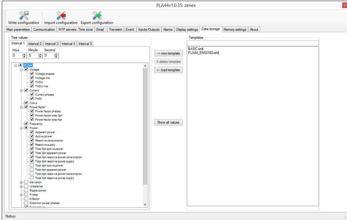
List of recorded parameters of all intervals can be saved as a template for further usage. There is also predefined template according the power quality norm EN 50160.
