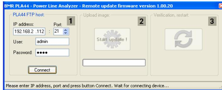
For the successful firmware update connect the PLA44 via Ethernet to PC where the Update software will run. Enter the IP address of the PLA44 and user name and password. Pressing button Connect will verify accessibility of PLA44 and prepare connection for firmware update start.
