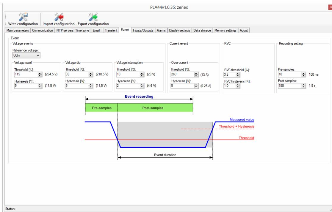
Common settings for absolute and differential transients is for the parameters used for tuning the transients detection and transients recording.
