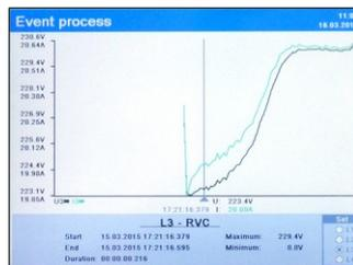
Moving the graph left or right use the buttons **▲** and **▼**. In order to select the phase or phases to be shown on graph press button **SET** and select the desired phase.
