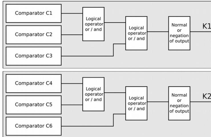
Comparators C1, C2 and C3 belong to the output K1 and comparators C4, C5 and C6 to output K2.
