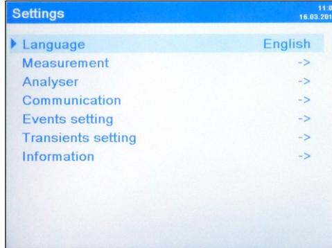
At main screen move to parameter **Settings** to open device various configuration sub-menu. Some of the device parameters and functions can be enabled and configured only by PC and software PMS.
