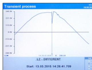
Waveform of transient event is possible be zoomed to the detail view by pressing the button **Fn (Zoom)**. The detailed zoom view can be moved forward and back by cursor buttons **▲** and **▼**.
