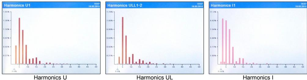
By pressing the button **SET** the cursor with value of particular harmonic is activated. Via cursor buttons the cursor pointer can be moved to display another harmonic details.
