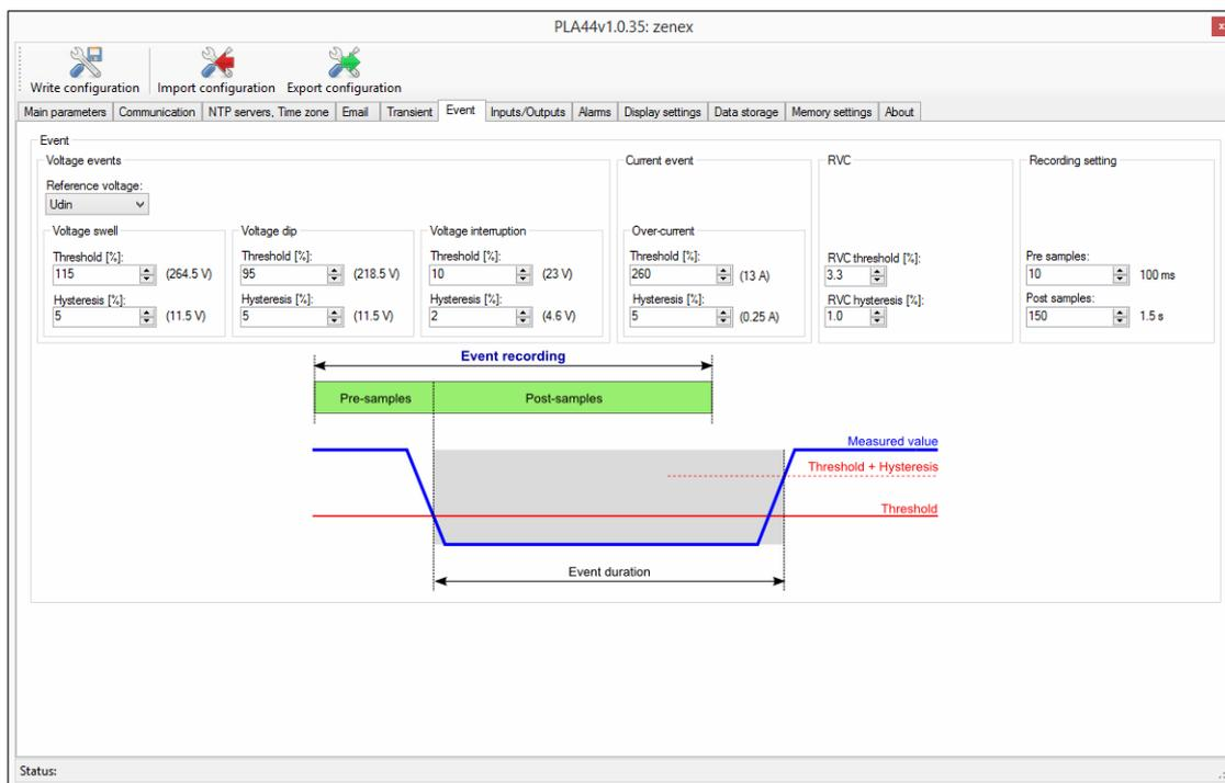
Events captured by PLA44 are fully adjustable by the parameters described in the table beneath.
