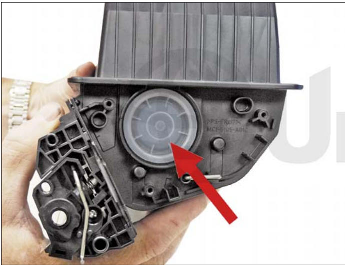
22. Remove the fill plug from the hopper.
