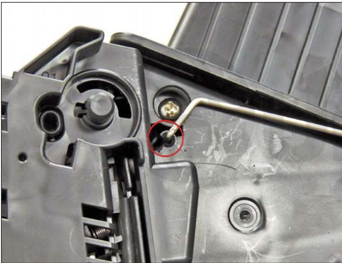
36. Install the metal bars from the drum cover on both sides of the cartridge. Place the bars in front of their slots, and press in place with a small screwdriver.
