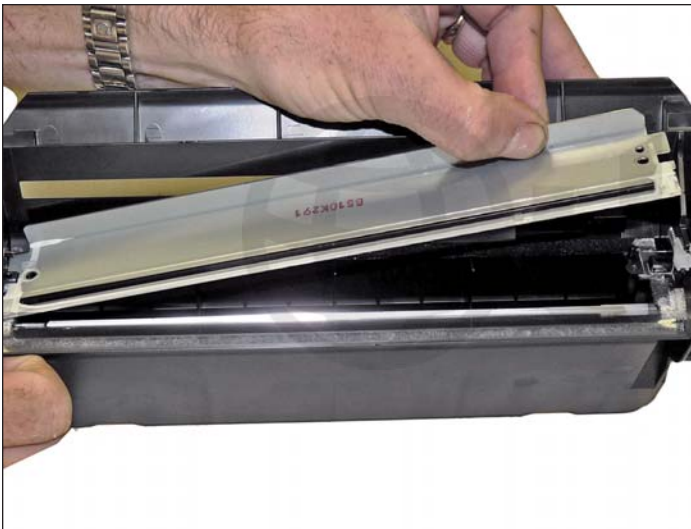
12. Note that there is no type of adhesive sealant on the wiper blade. There is just normal foam and felt seals under the blade.
