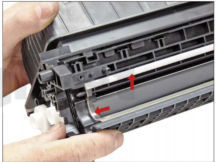
23. Note the magnetic seals on the magnetic roller sleeve, and the doctor blade's sealing foam. Make sure both are clean.
