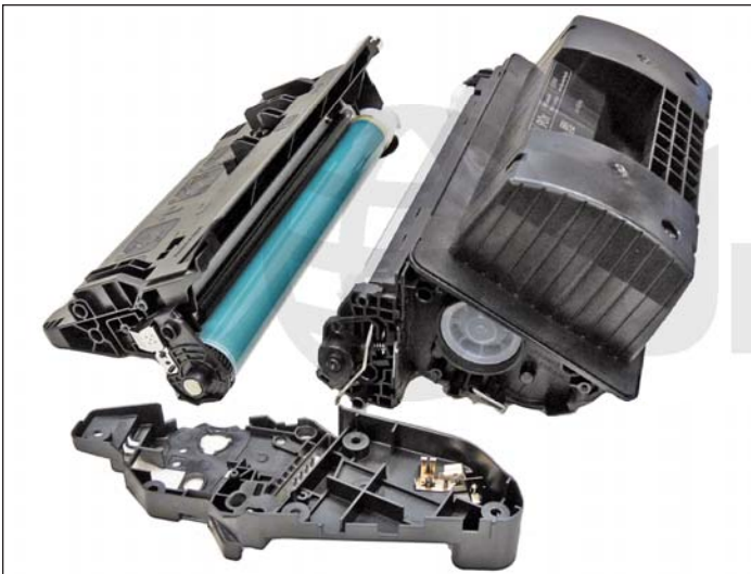
7. Remove the left side end cap. Both halves will come apart easily. Be careful not to damage the drum or the magnetic roller sleeve.
