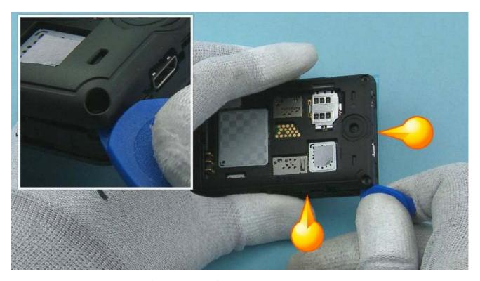
6) Start releasing the D-COVER from the top left corner with the SRT-6 to detach the two shown clips.
