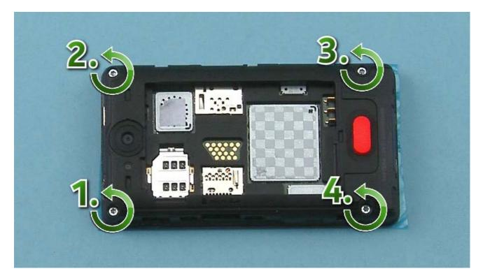
5) Unscrew the four Torx+ size 6 screws in the order shown.
