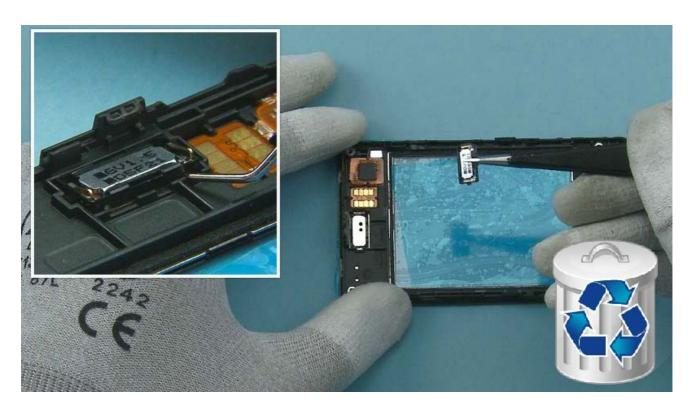
28) Release the EARPIECE with the dental tool and remove it with weezers. Do not use the EARPIECE again. Discard it.
