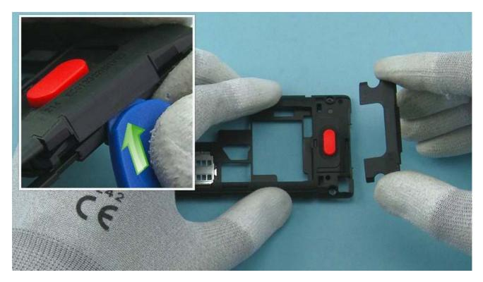
24) Push up to release the ANTENNA MODULE as shown with the SRT-6. Remove the ANTENNA MODULE.
