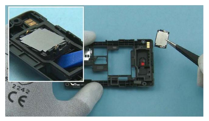
21) Use the SS-93 to release the IHF SPEAKER. Remove the IHF SPEAKER with tweezers.
