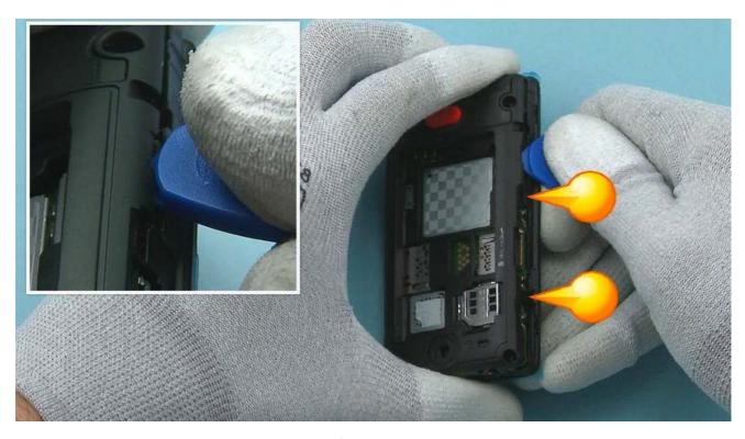
8) Then release the two clips on the right side of the device
