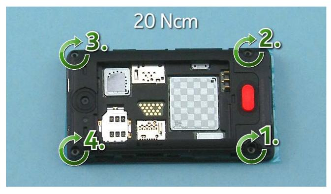
1) Fasten the four Torx+ size 6 screws in the order shown to the torque of 20 Ncm.
