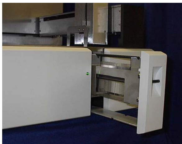
Figure 7-1: Loading a new Rack for Processing in the Load Drawer
