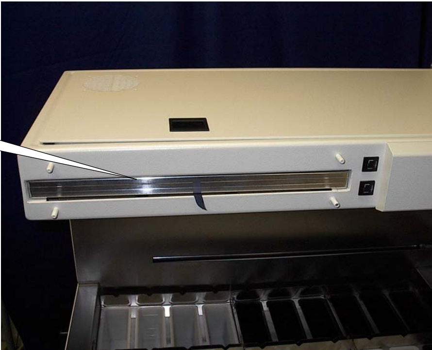
Figure 8-1: Charcoal Filter behind top left bezel
