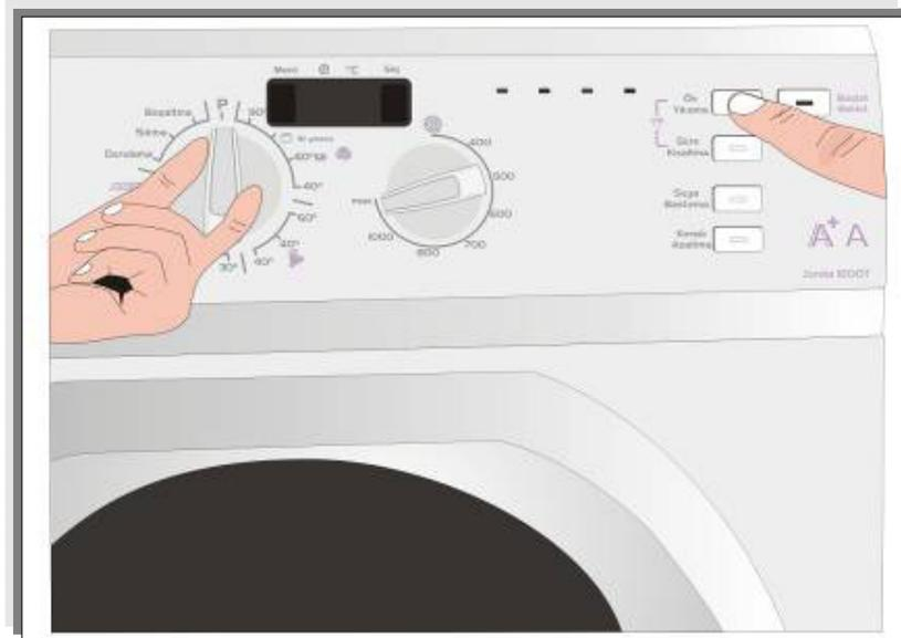
2) While pressing 1st Function button. Change the position of the knob to 1.
