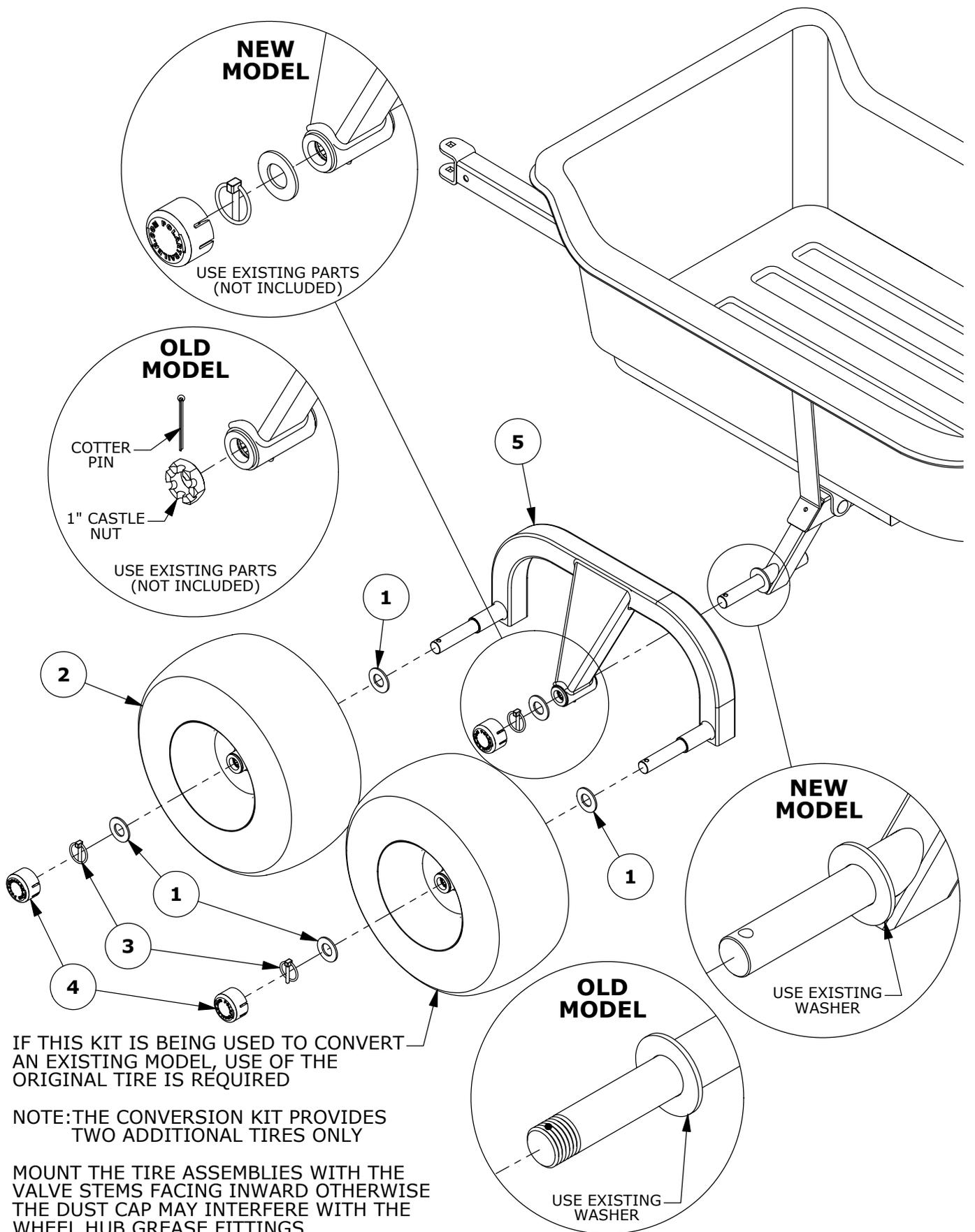
IF THIS KIT IS BEING USED TO CONVERT AN EXISTING MODEL, USE OF THE ORIGINAL TIRE IS REQUIRED
