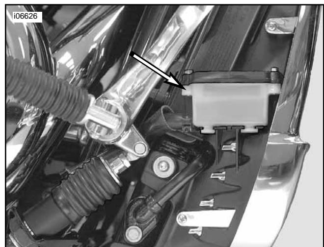
Figure 8. Fill 1/2 in. (12.7 mm) below Reservoir Gasket Surface (V-Rod)
