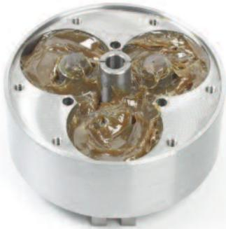
After setting 3 places, fill the space inside of the housing with Esso EP-1 High-pressure grade grease.
