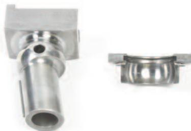
Also inspect the spherical portion of the actuator and the bearing race. If seizure is found on them, those surfaces would seem plated.
