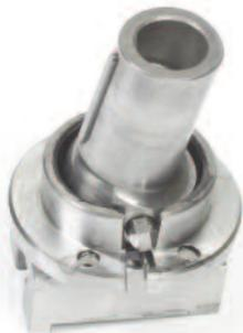
Left picture shows that the arm seal securely placed into the ditch of the bearing race.
