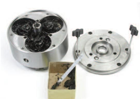
Left picture shows the back plate is removed from the chuck.
