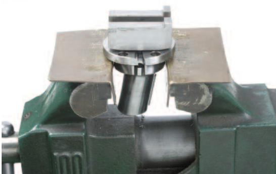
Put together the bearing race by a vice as making sure that the restrictor pin can fit into it well. (Refer to next page)
