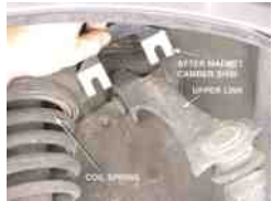
FIGURE 52.44 An aftermarket camber shim can be added to change the front camber on this Honda.
