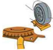
FIGURE 52.14 The protractor scale on the front turn plates allows the technician to test the turning radius by turning one wheel to an angle specified by the manufacturer and observing the angle of the other front wheel. Most newer alignment machines can display turning angle based on sensor readings, and therefore the protractor scale on the turn plate is not needed or used.
