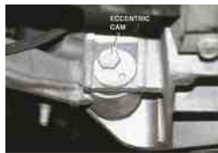
FIGURE 52.21 The rear camber is adjustable on this vehicle by rotating the eccentric cam and watching the alignment machine display.
