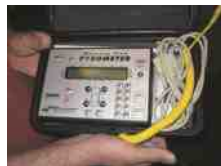
FIGURE 52.46 A typical tire temperature pyrometer. The probe used is a needle that penetrates about 1/4 inch (7 mm) into the tread of the tire for most accurate readings.
