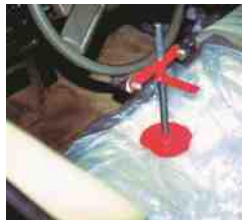
FIGURE 52.37 Many procedures for setting toe specify that the steering wheel be held in the straight-ahead position using a steering wheel lock, as shown. One method recommended by Hunter Engineering sets toe without using a steering wheel lock.
