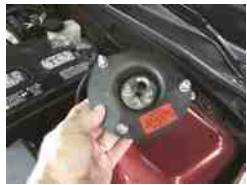
FIGURE 52.45 An aftermarket kit for this Ford is installed at the top of the strut tower and allows more camber and caster adjustment than is possible with the factory adjustment.
