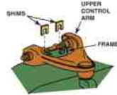
FIGURE 52.33 The general rule of thumb is that a 1/8 inch shim added or removed from both shim locations changes the camber angle about 1/2 degree. Adding or removing a 1/8 inch shim from one shim location changes the caster by about 1/4 degree.
