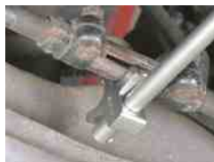
FIGURE 52.40 Special tie rod adjusting tools should be used to rotate the tie rod adjusting sleeves. The tool grips the slot in the sleeve and allows the service technician to rotate the sleeve without squeezing or damaging the sleeve.
