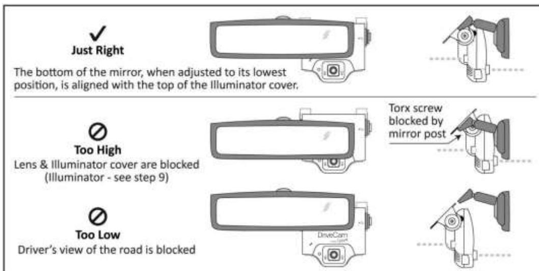
**Mounting Options:** Refer to the **DriveCam Mounting Guidelines (DRC 340)** if you're installing in a vehicle without a standard rear view mirror. The document provides additional details and diagrams about VER mounting in various vehicle types, including instructions for using the **Extended (Bulkhead) Bracket** and **RAM-Mount (Articulating) Bracket**. Government restrictions regarding the mounting of objects on the vehicle windshield and U.S. DOT exemptions are also covered.
