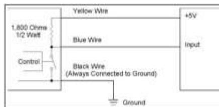
**NOTE:** With the yellow (supply) wire connected to a switched voltage source and the UM05's OUT switch set to NORM HI, the blue wire will go low whenever the voltage is turned off even though there is no event. If the electronic device requires a voltage other than the normal vehicle voltage (i.e. a +5V level) and that voltage is available at the device, simply connect the yellow wire to the voltage source.
