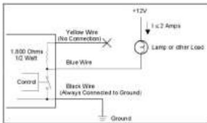
In example 2, because we are switching the ground wire, operation of the device may seem backwards.
