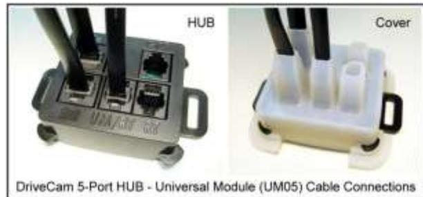
**A)** Remove the shell from the HUB. Refer to the connection diagram on page 3 to determine which cables plug into which ports on the HUB.
