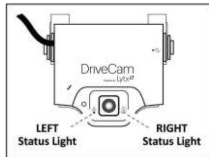
**Errors:** If the status lights **did not light at all**, check the wiring and fuses.
