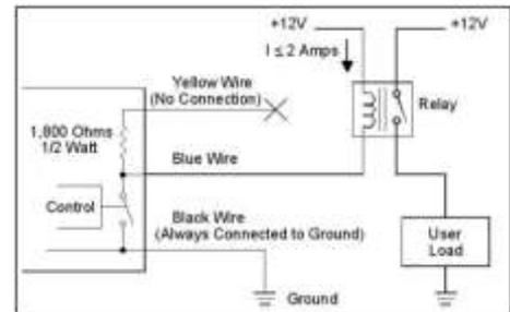
**Example 4: Triggering a secondary electronic device that needs more drive current**
