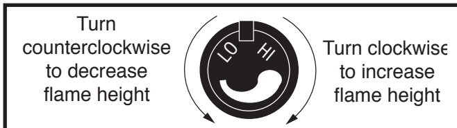
Fig. 41 Flame adjustment knob for Honeywell valve.
