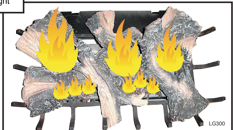
Fig. 44 Correct burner flame appearance.
