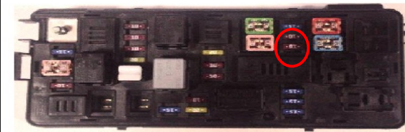
Location of 15 Amp LPG Minifuse in IP Junction Box.
