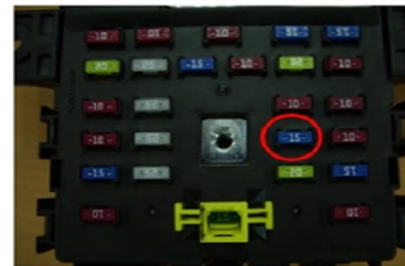
Location of 15 Amp LPG Minifuse in IP Junction Box.
