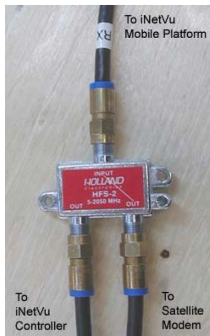
Fig. 19: RF-Splitter Connections
