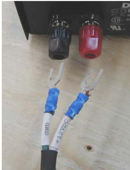
*Fig. 5: Connecting 12VDC Power Cable to DuraComm® LP-18 Power Supply*
