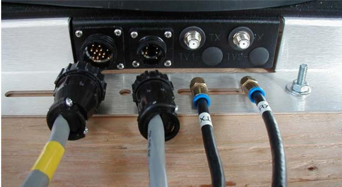
*Fig. 18: From left to right: Sensor Cable, Motor Control Cable, Tx and Rx RG6 Coaxial Cables*
