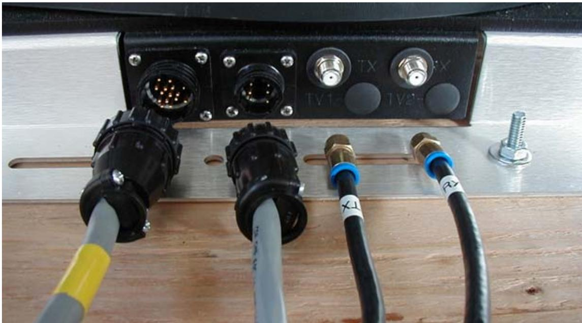
Fig. 4: From left to right: Sensor Cable, Motor Control Cable, Tx and Rx RG6 Coaxial Cables
