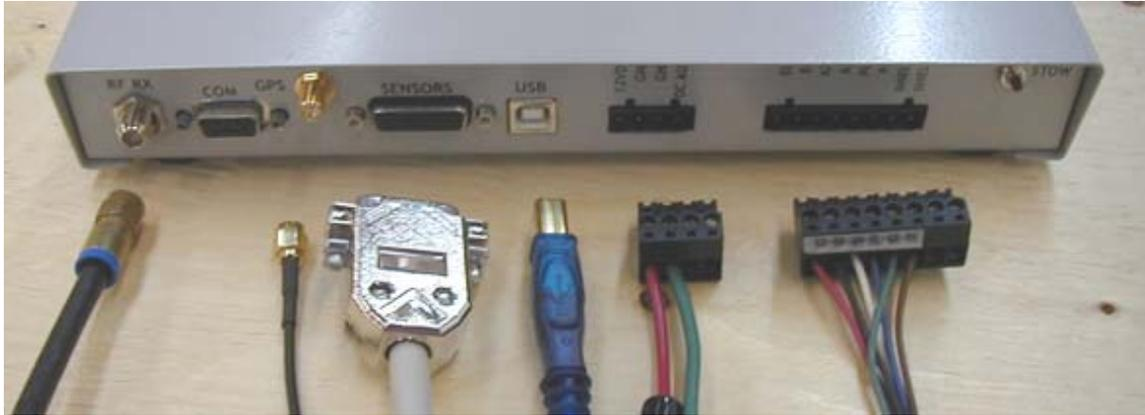
Fig. 3: From left to right: RG6 Coaxial Cable, GPS Antenna, Sensor Cable, USB Cable, 12VDC Power Cable, Motor Control Cable
