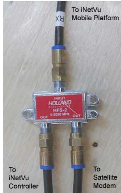
Fig. 6: RF-Splitter Connections
