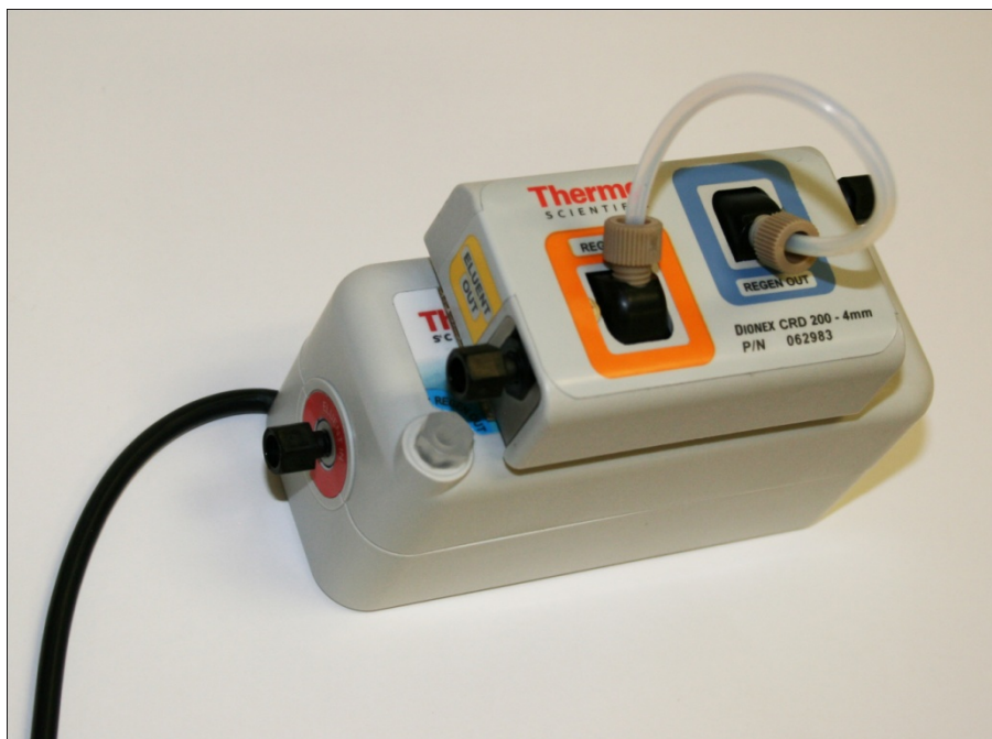
Figure 6 Dionex CRD 200 Installed on Suppressor
