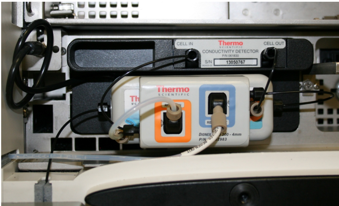
Figure 8 Dionex CRD 200 Installed in the System
