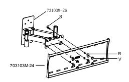
6. Put the TV or LCD panel onto the plate using the hooks. Once positioned, tighten the lower screws shown to lock the rails into place.
