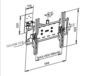
The viewing angle can be adjusted by loosen or tighten 703103M-25-2.
