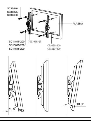
5. Mount the plate to the arm assembly. Level the plate and tighten the mounting hardware.
