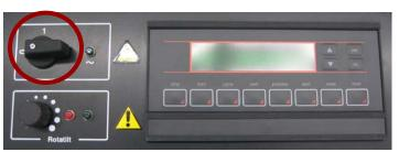
Turn the cooling water switch to OFF – Do not adjust the flow rate.
