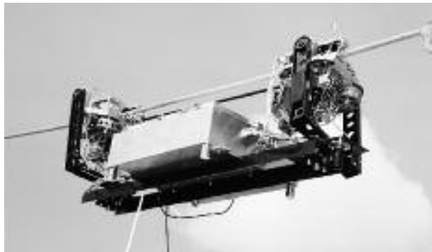
“Ti,” a 140-lb. robot being developed by the Electric Power Research Institute, hangs gondola-style from bulk power lines and rides slowly from tower to tower, monitoring the condition of the lines. Robots like Ti seek to prevent power outages. Photograph provided by Electric Power Research Institute
