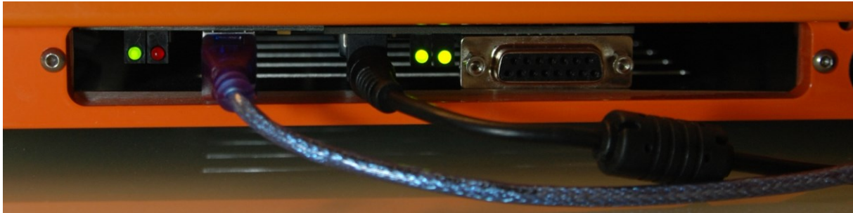
(left-to-right direction. USB module LED 1, control board LED 2 and LED 1)
