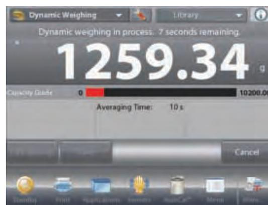
After the cycle ends, remove the specimen and the balance returns to the Home screen automatically (after a 10-second delay).
