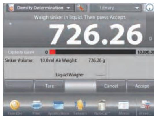
Once the necessary weights have been determined, the density of the Liquid sample is displayed in **g/cc** (along with the weight in air, weight in water) on the Application screen.
