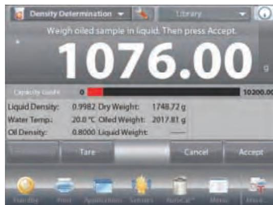
Once the necessary weights have been determined, the density of the sample is displayed in **g/cc** (along with the weight in air, un-oiled and oiled, and weight in water) on the Application screen
