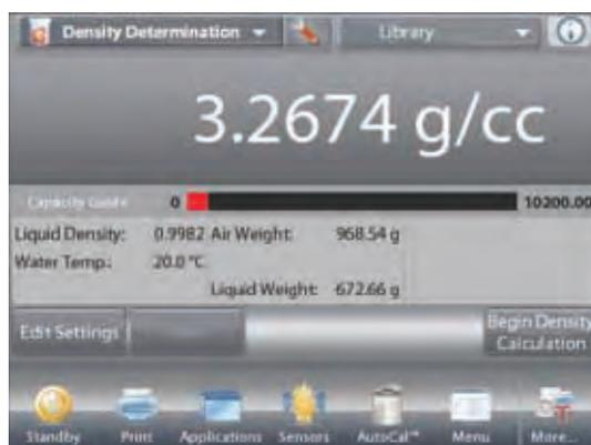
Once the necessary weights have been determined, the density of the sample is displayed in **g/cc** (along with the weight in air, weight in water) on the Application screen.
