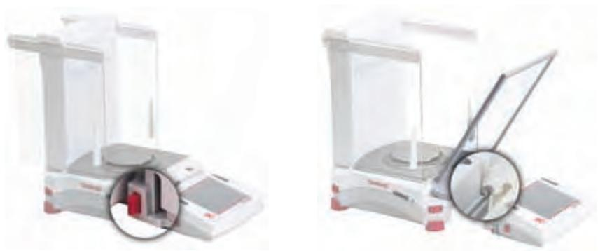
Press button to separate Terminal from Base. Seat panel's hooked ends in base. Swing panel to vertical position.
