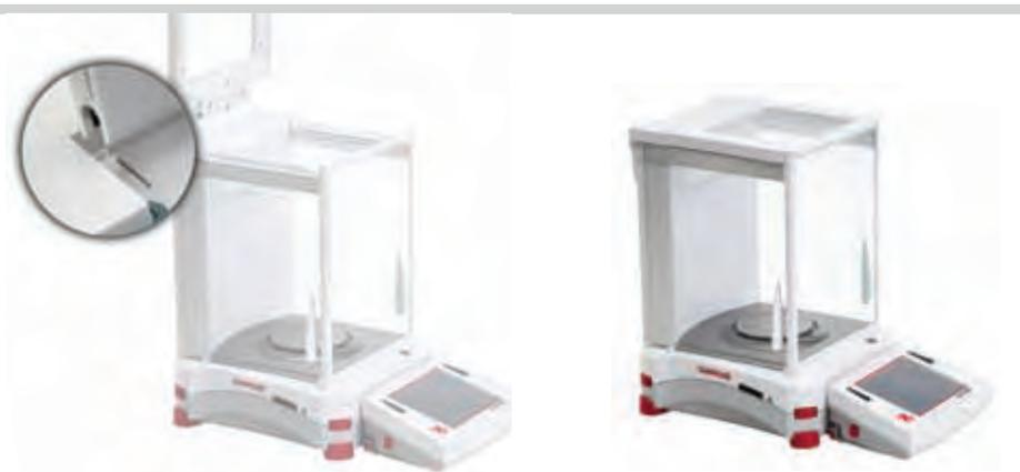
Insert Top Door's hooked ends in grooved pegs. Press gently to seat. Check for smooth movement. Close door.
