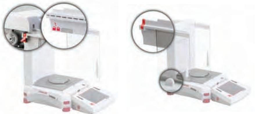
Position glass door to slide. Open lock tab (top); insert in top groove and slide inside bottom groove. Close lock tab.
