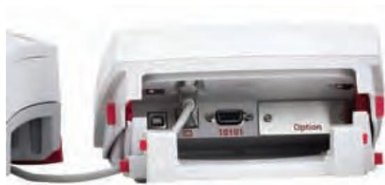
Interface connections on back of Terminal.
