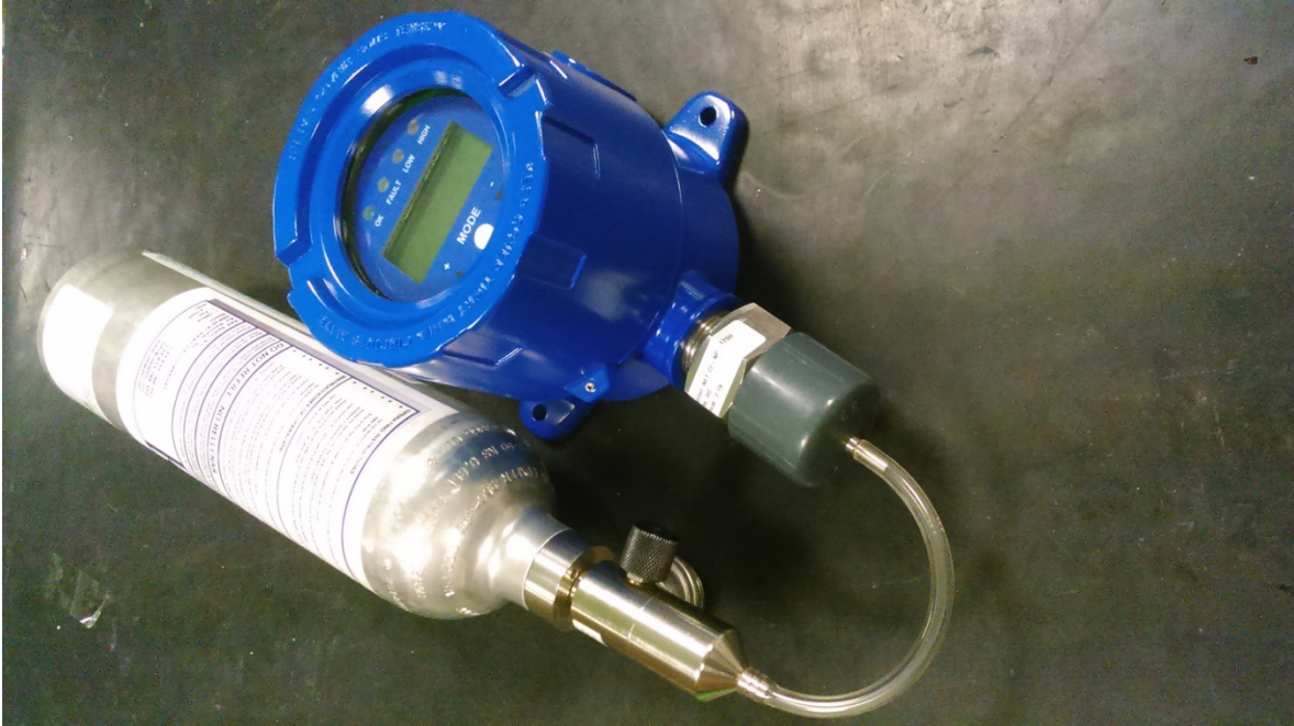
Sensotox 2 connected to a calibration gas cylinder with an adapter.
