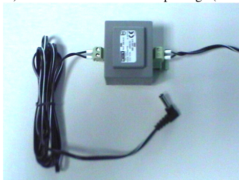
FIGURE 2.4: FEEDING ISOLATION TRANSFORMER 24V AC – 24 V AC
