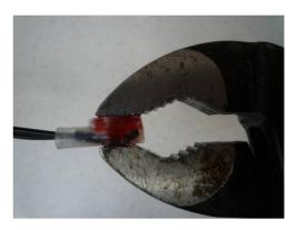
You will see that a gel, which is located in the red cap, will be injected in the cable insertions.
