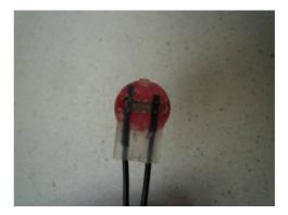
After verifying that the cable is still in good position, you can put the Scotchlok<sup>TM</sup> connector in the tube.
