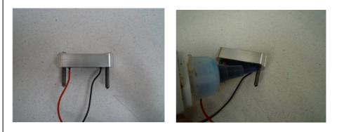
After applying the glue, turn the screws back to approx this situation:
