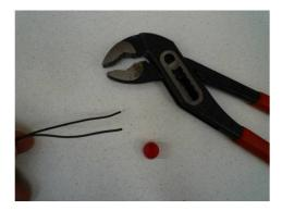
Insert the trimmed wire ends into the connector. Do not strip the wires. Make sure all wires are inserted past the metal element to the back wall of the connector.
