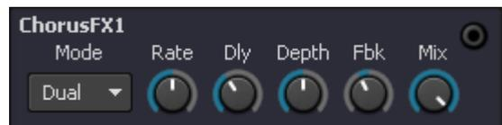
**Dual Mode** : In this mode there are 2 chorus voices added to the input signal. This is a typical “stomp box” type chorus effect.
