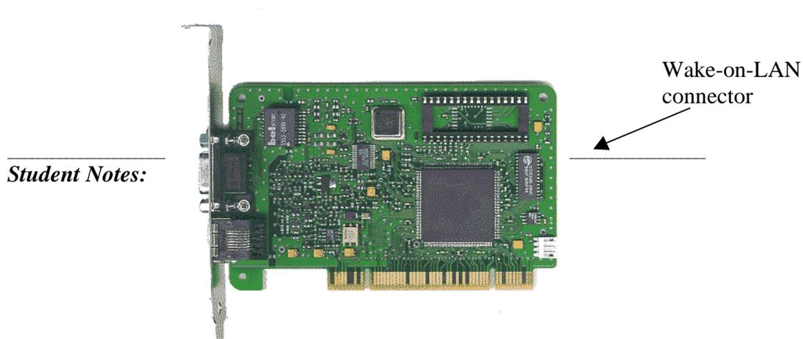
**Figure 23. Smart 16/4 PCI Ringnode Mk3 (Wake-on-LAN)**
