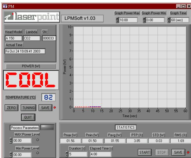
Whenever the temperature of detector head is above its limit, this will be displayed as a *COOL* alarm (red). In this cases, switch the laser off and cool the head taking care not to contaminate the absorbing surface. Note: occasional dirt or contamination of absorbing surfaces may compromise system performance both regarding damage thresholds and measurement precision.
