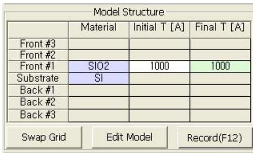
A screenshot of the 'Model Structure' dialog box. It contains a table with columns: Material, Initial T [A], and Final T [A]. The rows are: Front #3, Front #2, Front #1, Substrate, Back #1, Back #2, and Back #3. The 'Front #1' row is highlighted in blue, showing 'SIO2' for Material, '1000' for Initial T, and '1000' for Final T. The 'Substrate' row shows 'SI' for Material. Below the table are three buttons: 'Swap Grid', 'Edit Model', and 'Record(F12)'.
