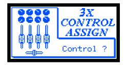
3. Now move the control you want to assign (ie: any fader, knobs, switch button, cross-fader, joystick, infrared axis or automation potentiometers). You automatically enter the control assign menu.
